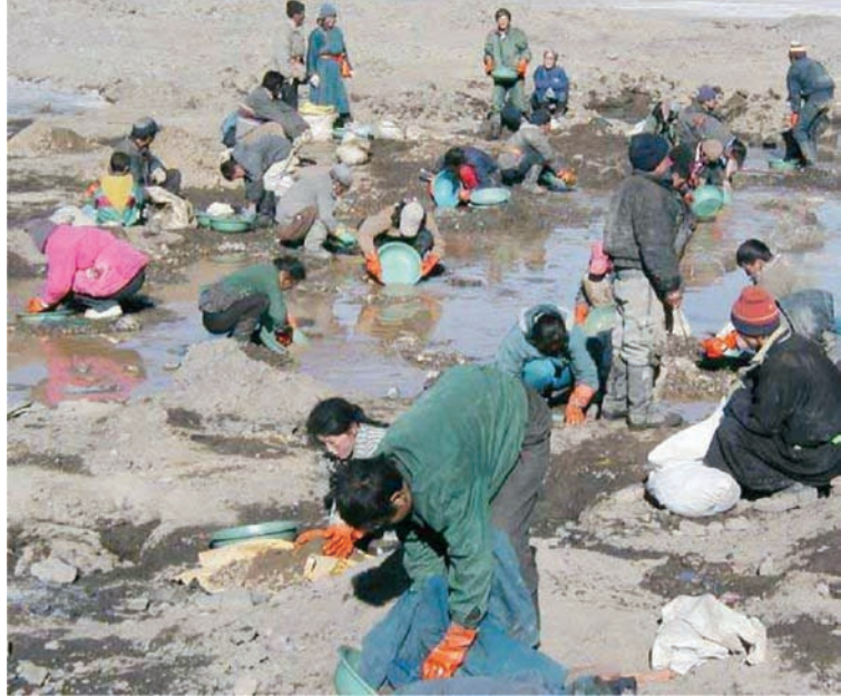
A large group of ninjas, mostly women and teenagers, using green plastic kitchen bowls for “bowling” pay-gravel in a pool of spring meltwater. The pay gravel is defrosted “permafrost.” The pay gravel is carried here in old flour sacks and several handfuls are put in a bowl for bowling. All are wearing warm clothing and rubber kitchen gloves. (Image: William Murray of Murray Harrison Ltd.)
