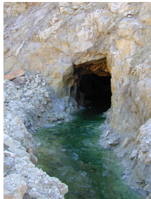
Dark greenish-black drainage from a mine adit indicative of ferrous iron ( Fe^{2+} ) (Gilt Edge, South Dakota) (Photo taken by S. Shaw, 2000).
