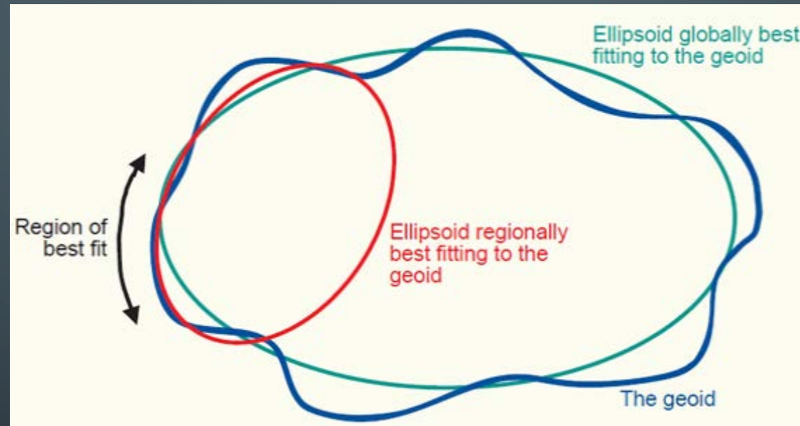
A globally best fitting and a regionally best fitting ellipsoid (shapes exaggerated)
